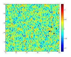
Realization of random medium with strength of fluctuation  $\sigma_0=3\%$  and correlation length half of wavelength
