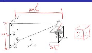
Configuration: range is  $100\lambda_0$ ; array size is between  $100\lambda_0$  and  $200\lambda_0$  with transducers half of wavelength apart; target area is box of length  $20\lambda_0$  with half of wavelength resolution
