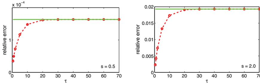
FIG. 5.3. Relative error  $E_{rel}(\tau, s)$  versus lag time  $\tau$  (dashed line) compared to the upper bound  $\delta^2$  given by Theorem 4.2 (solid line) for  $s = 0.5$  (left) and  $s = 2$  (right).
