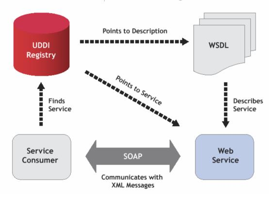
The Web service architecture is based upon the interactions between the service application that is looking for and invoking an interaction with a service stry owner of the services
