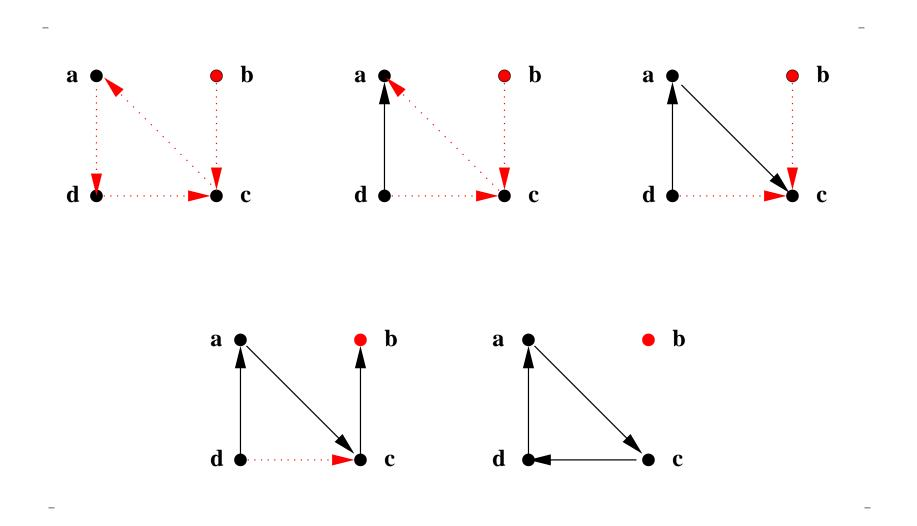
Site c believes  $\mathcal{M}$  is in d. It now forwards pending com. msg. to d The tree structure is destroyed: we have a CYCLE.
