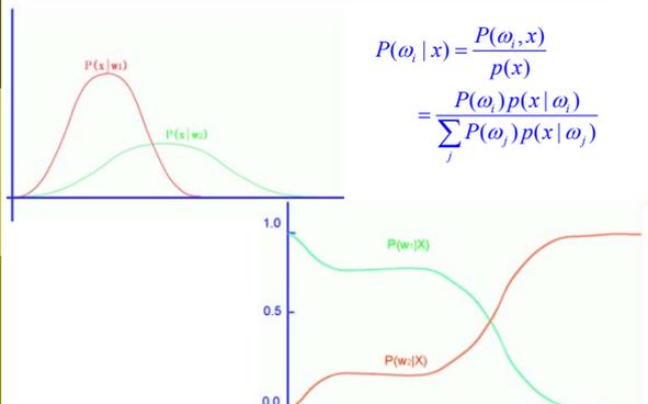
$$P(\omega_i|x) = \frac{P(\omega_i, x)}{p(x)} = \frac{P(\omega_i)p(x|\omega_i)}{\sum_j P(\omega_j)p(x|\omega_j)}$$
