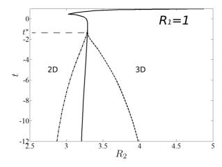
Figure 5: Phase diagram for the planar anchoring condition on both inner and outer spheres.
