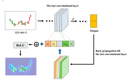
Figure 10. A schematic illustration of Grad-CAM.
